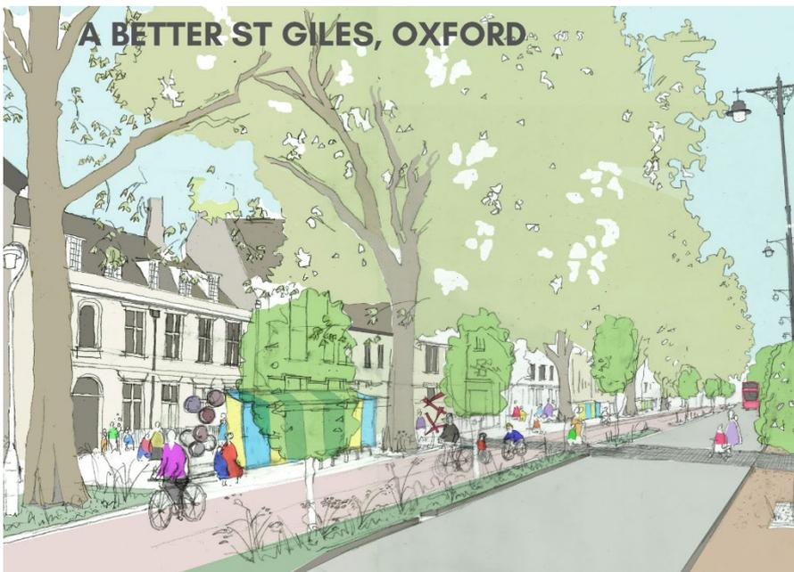
Figure 3: Space reallocated in St Giles to provide a segregated cycle track, kiosks and sculptures in the old parking area and a pedestrian crossing. Looking north and west
